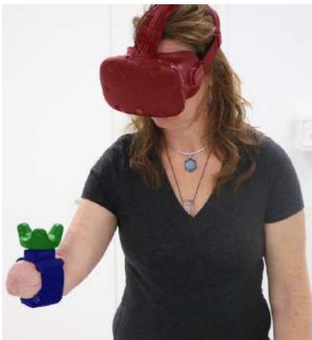
Figure 1: A subject wearing the EMG arm-cuff (blue), with the attached tracking puck (green). The immersive environment is rendered through the virtual reality headset (red).
